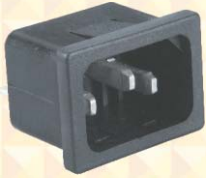
NPS - 1 (SNAP MOUNTING) 10A, 250 V AC Cut out size: 19.8 mm X 27.4 mm For 1.5 / 2.0 mm Panel thickness
