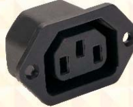
EMO-21 (SCREW MOUNTING) 10A, 250VAC Cut out size 25 mm x 32.5 mm
