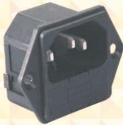
NPS - 3F (SCREW MOUNTING) 10A, 250 V AC Cut out size: 27.3 mm X 31.2 mm
